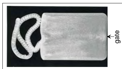
Figure 3.10 Short-shot moulding showing jetting (source: Akay (1992))
