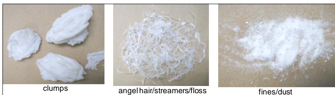
Figure 3.3 Types of degradation in delivery/conveying
