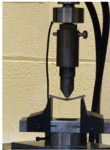
Figure 6.14 A specimen tested in 3-point bending
