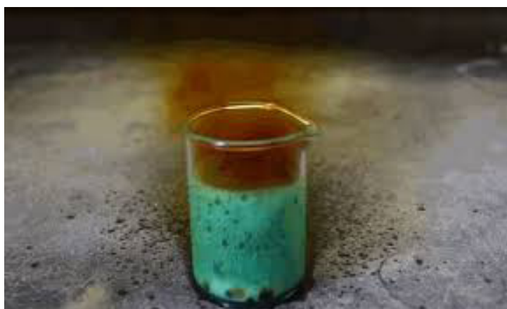
Copper dissolving in concentrated nitric acid [Exploratorium]
