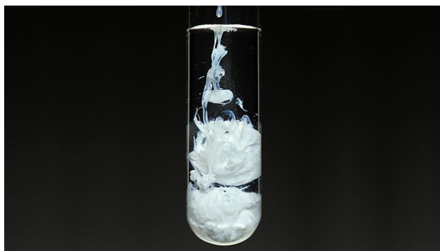
Adding silver nitrate to sodium chloride [BBC]
