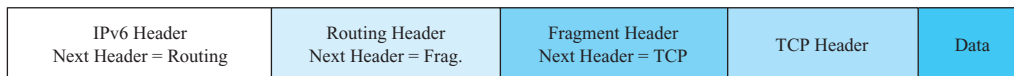
(c) IPv6 header followed by a routing header and a fragment header
