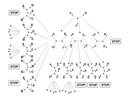
Figure 5.11: Example for constructing trees with the brunch-and-bound method. Trees with STOP mark do not possess successors because their tree length exceeds the upper bound.
