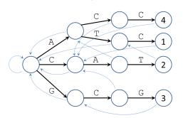
Figure 3.8: Also Corasick finite state machine for DNA string matching. Blue arrows are failure links, that point to the node where the algorithm jumps to if it hits a mismatch. Using failure links the algorithm does not have to start at the root each time.
