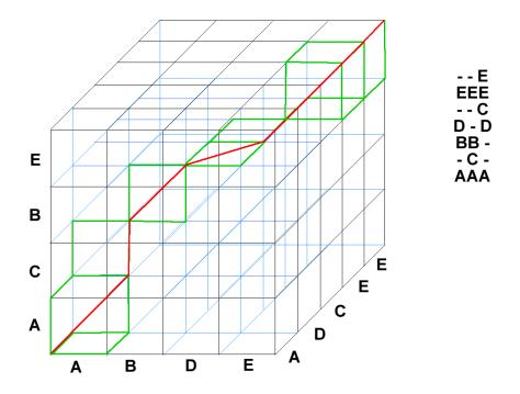
Figure 4.5: Cube for aligning three sequences. Each path from the lower, left, front to the upper, right, back through the cube is an alignment of three sequences.
