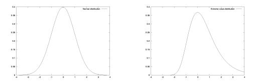
Figure 3.10: The density functions of the normal distribution (left) and the extreme value distribution (right).
