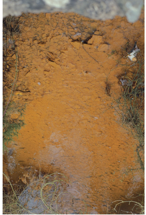
Plate 5.2 Crusts of iron oxide (goethite) coating stream bed. Drainage from Parys Mountain, copper mine Anglesey, UK. Photograph courtesy of J. Andrews.
